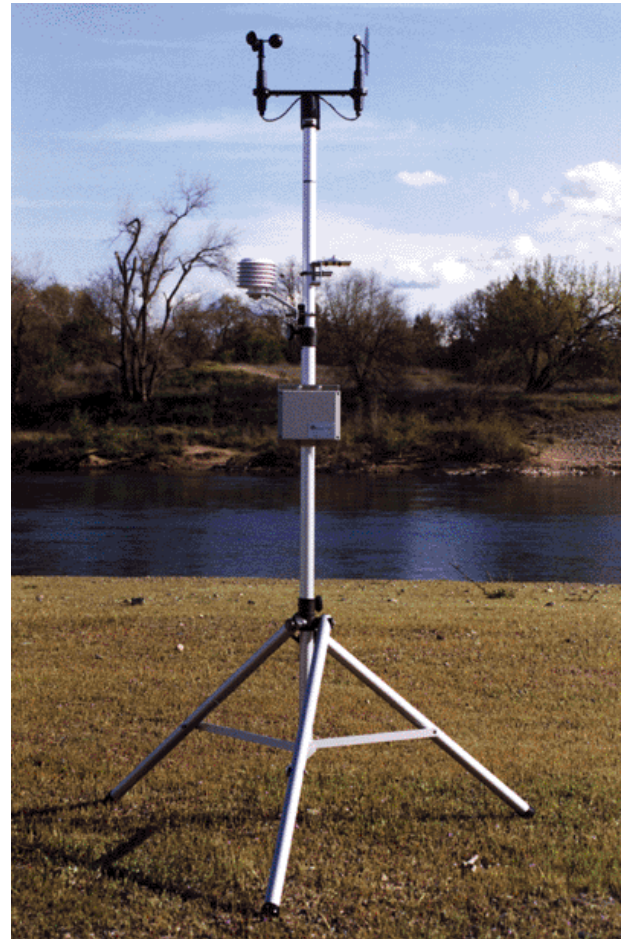
The Micro Weather Pro™ can be deployed using this lightweight 9' aluminum tripod, a 3m steel tripod, or a 30' tower. Anchoring stakes are available for tripod stability.
